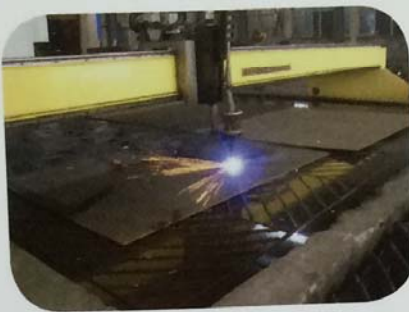
Three units of Large Power Plasma Cutting Enssure clean and efficient Steel cuting.
